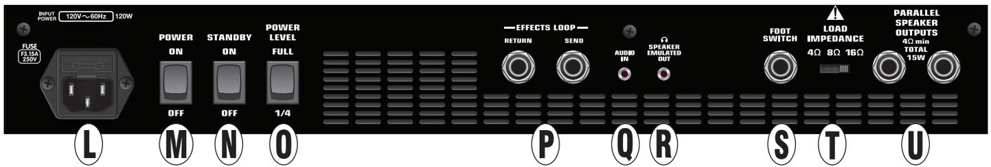
**L. POWER INPUT:** Connect included power cord to amplifier here, in accordance with the voltage and frequency ratings listed on rear panel of amplifier. Power input's integral fuse holder houses a spare fuse. Replace only with a fuse of the same current and voltage rating as printed on the back of the amplifier.
